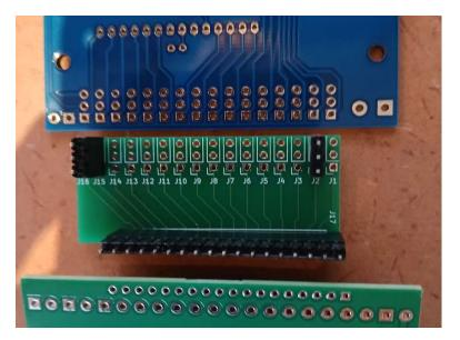
5. Now the Dupont pins can easily be soldered on the DCCNext.
