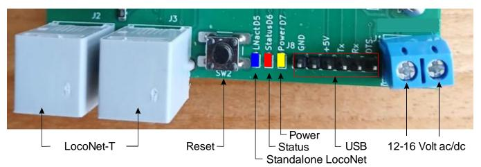
The USB interface (CH340) must be connected to an USB port on the PC. This also allows the LocoNext to be supplied with power. This interface must be ordered separately!
