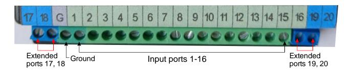
The *Ground* must be connected to the ground of the module that provides the input signals.
